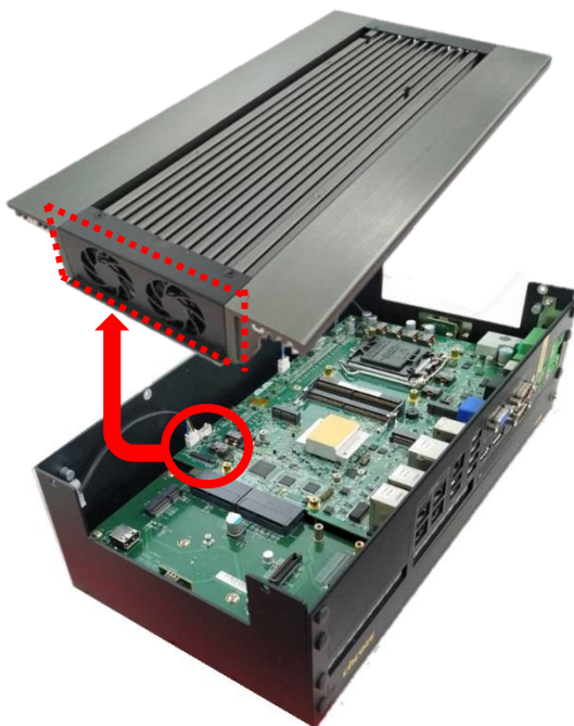
POWER1 (FAN OUT Control)
